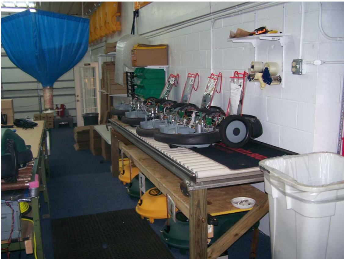
Holding conveyor - for pending service bots
