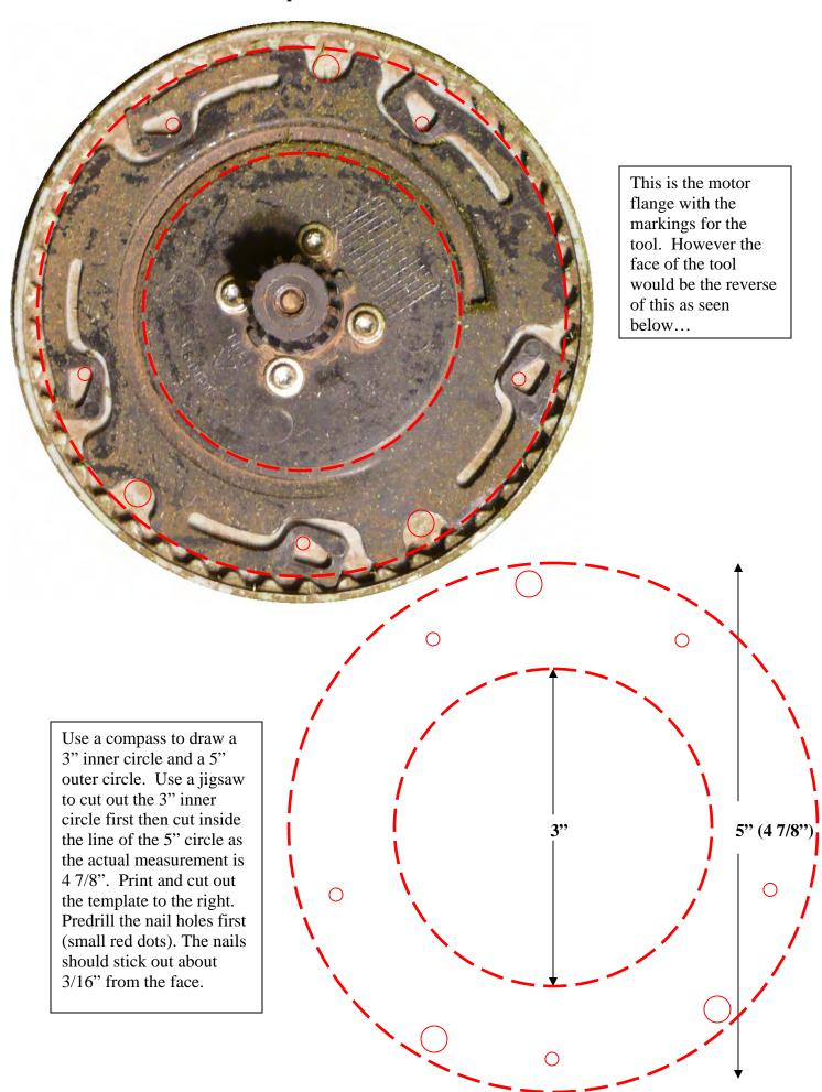
Scrap 3/4" plywood and 5 finish nails. Outside diameter 4 7/8"- Inside diameter 3". The tool only goes on one way... for some reason due to spacing it won't connect correctly unless you line up the notch markings even though the spacing looks equidistant.
