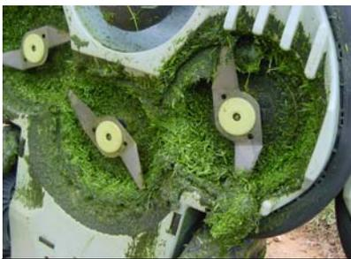
Clippings and debris in mowing deck
