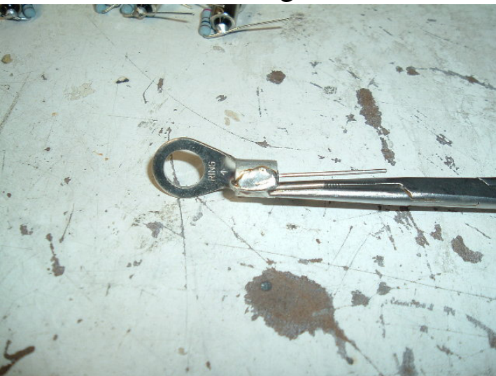
11. Solder it with >60W solder iron
