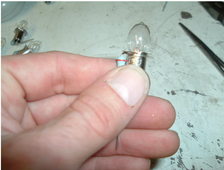
3. Wrap Lead Round Bulb
