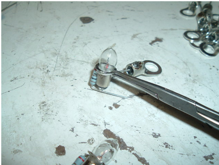
15 Solder '+' Ring to Lamp
